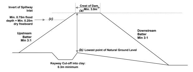
Note: The cut-off trench is required to be taken down a minimum of 300 mm into impervious soil and backfilled with good quality clay that is thoroughly compacted.
