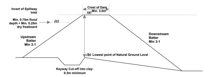
Note: The cut-off trench is required to be taken down a minimum of 300 mm into impervious soil and backed filled with good quality clay that is thoroughly compacted.
