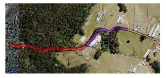
The purple section is a 350m length of Lawless Road not currently maintained by Council. The section in red is a 380m length of unformed roadway that is currently a Crown Road.
